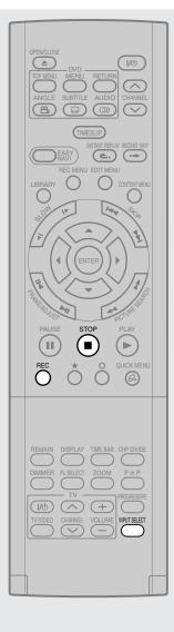
Press INPUT SELECT repeatedly so that "L-1," "L-2," or "L-3" appears on the front panel display, corresponding to the input in which the device is connected.
